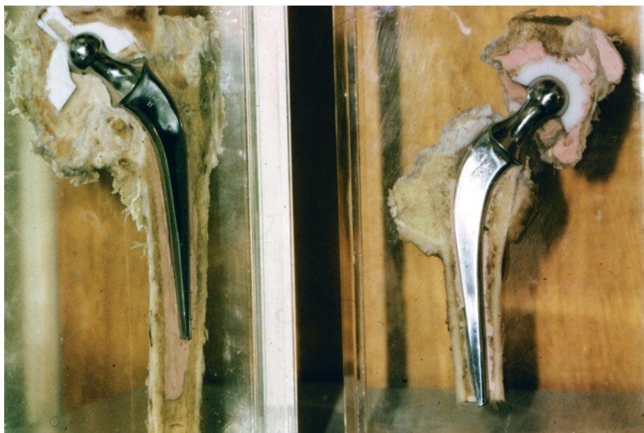
Figure 4 Two samples from autopsies. On the left, a Teflon acetabular cup worn out after some years of use. Note vertical direction of wear track. On the right, the future-oriented prosthesis with an acetabular cup made of ultra-high molecular-weight polyethylene first used by Charnley in 1962. The picture was taken in 1967 when Sudmann visited Charnley. Photo: Einar Sudmann
