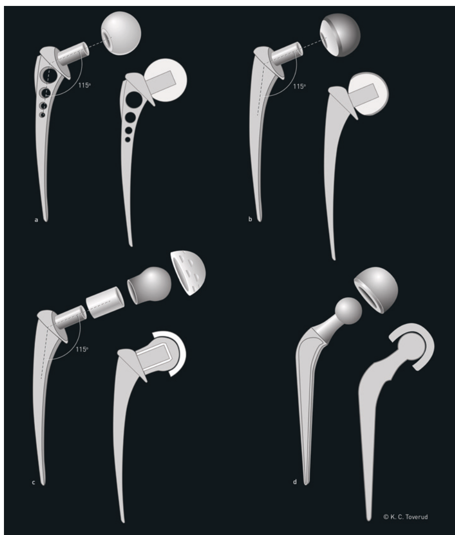
Figure 3 a) Christiansen's hemiprostheses as used in the period 1965–67. A loose femoral head articulates with a cylindrical trunnion on the stem of the prosthesis, the trunnion bearing. To achieve a lasting fixation in the femoral canal, the stem of the prosthesis had several perforations, similar to the stem of an Austin Moore hemiprostheses. The perforations were intended to permit ingrowth of bone tissue to fixate the stem permanently to the bone. The angle between the head and the stem is 115°. The femoral head was initially made of Teflon, from 1967 of polyethylene. b) Christiansen's hemiprostheses as used from 1968. The loose femoral head, with a steel coating added by the Polaris factory in Sandnes, was initially made of polyethylene, later of Delrin. The stem is smooth for fixation with cement. c) Christiansen's total prosthesis as used from 1970. The relatively large metal femoral head articulates on the inside against a sleeve of Delrin and on the outside against a relatively thin-walled artificial acetabular cup made of Delrin. The acetabular cup has small indentations on the outside to enable adherence of the cement. The stem is smooth for fixation with cement. d) A modern Charnley-Hastings hemiprostheses with a loose femoral head of polyethylene with a steel coating. The femoral head articulates against a standard Charnley stem with a small head, and the steel coating – as in all other hemiprostheses – against the joint cartilage in the acetabulum. In 1969, Christiansen was granted a US patent for this kind of «ball-and-socket joint», bipolar hemiprostheses in 1969.
